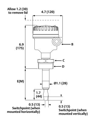
A. Cable Entry M20x1.5 or  $^1$ /2-in. ANPT B. Cable Entry M20x1.5 or  $^3$ /4-in. ANPT C. 2.6 (65) A/F Hexagon
