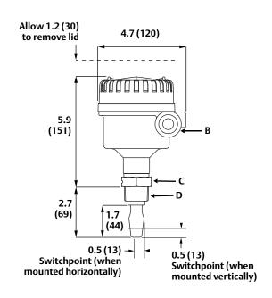
A. Cable Entry M20x1.5 or <sup>1</sup>/<sub>2</sub>-in. ANPT B. Cable Entry M20x1.5 or <sup>3</sup>/<sub>4</sub>-in. ANPT C. 1.6 (40) A/F Hexagon
