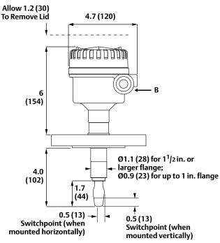
A. Cable Entry M20x1.5 or  $^{1}$ /2-in. ANPT B. Cable Entry M20x1.5 or  $^{3}$ /4-in. ANPT
