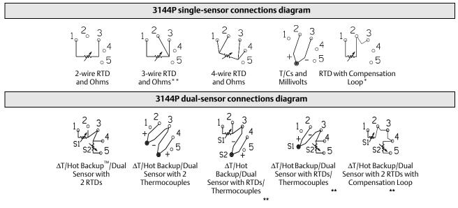
\* Transmitter must be configured for a 3-wire RTD in order to recognize an RTD with a compensation loop.
