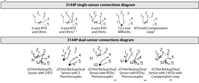
\* Transmitter must be configured for a 3-wire RTD in order to recognize an RTD with a compensation loop.
