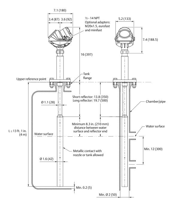
Figure 16. Rigid Twin Lead Probe
