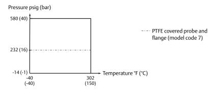
Final rating may be lower depending on flange, material of construction, and O-ring selection. Table 4 on page 38 gives the temperature ranges for standard tank seals with different O-ring materials.
