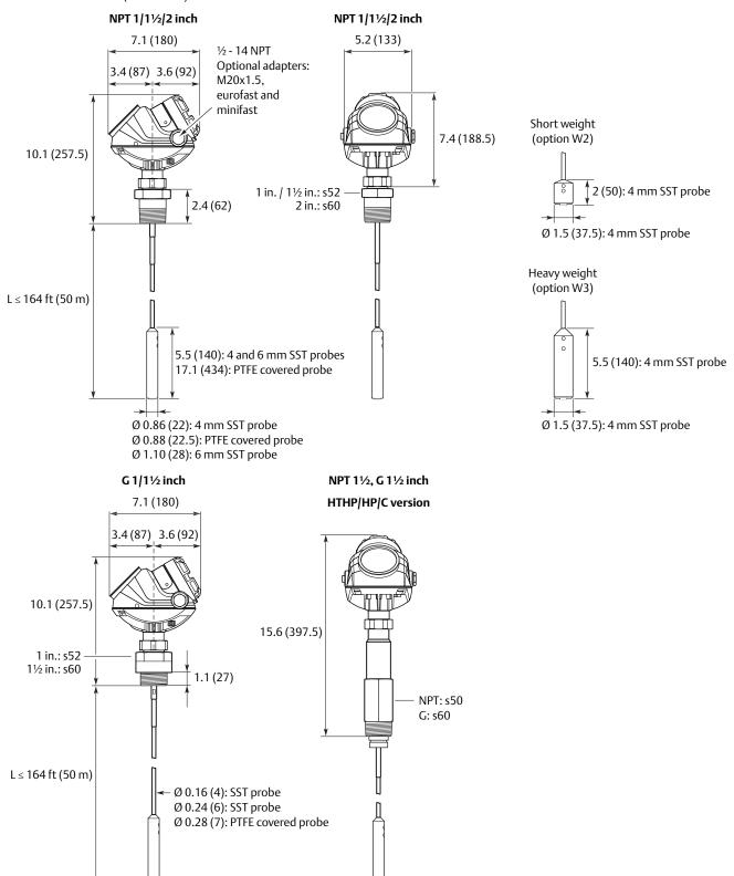
Figure 13. Coaxial Probe with Flange Connection
