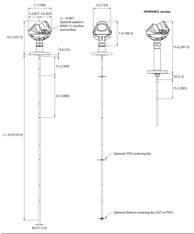
Figure 8. Segmented Rigid Single Lead Probe with Threaded Connection
