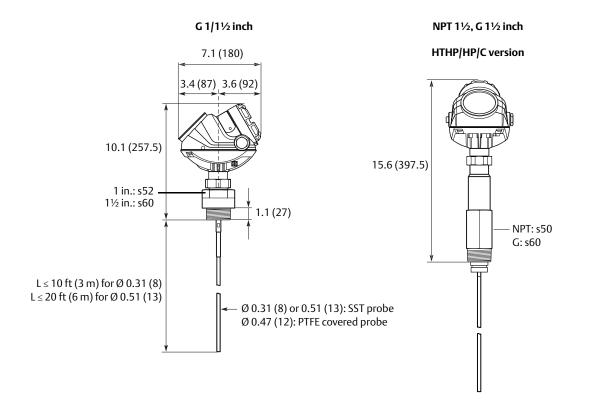
Figure 7. Segmented Rigid Single Lead Probe with Flange Connection
