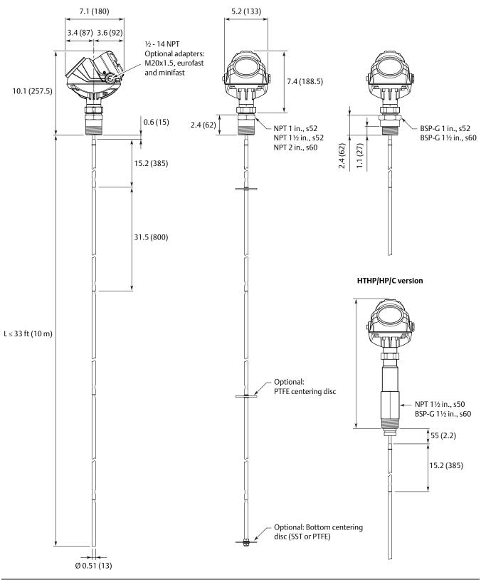
Figure 9. Single Rigid Vapor Probe for 2-in. Chambers
