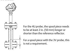
Always ensure that there are no disturbances from inlets etc close to the reference reflector end when using probe type 4U.
