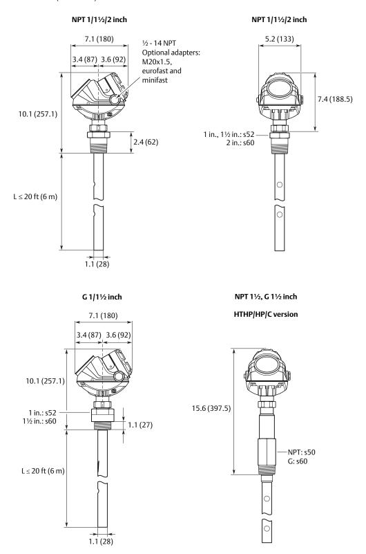
Figure 15. Integrated Still Pipe Vapor Probe for 3-in. Chambers and above
