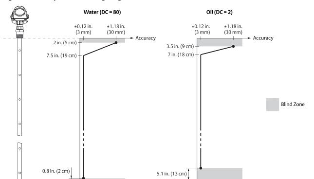
Figure 2. Accuracy Over Measuring Range for Coaxial Probe
