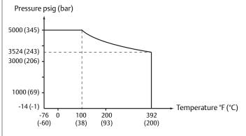
Final rating may be lower depending on flange selection and material of construction.
