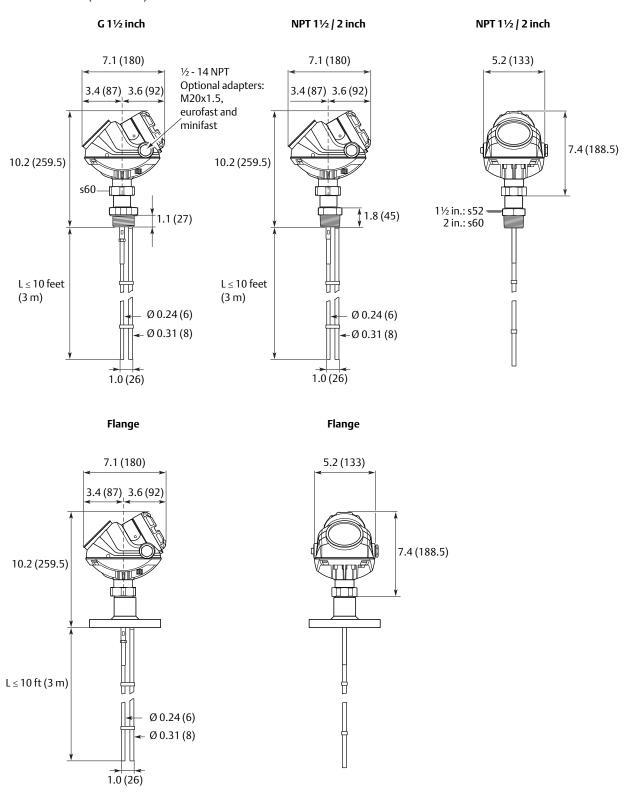
Figure 17. Flexible Twin Lead Probe
