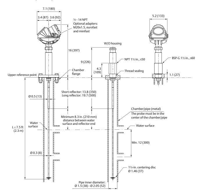
Figure 10. Flexible Single Lead Probe with Flange Connection
