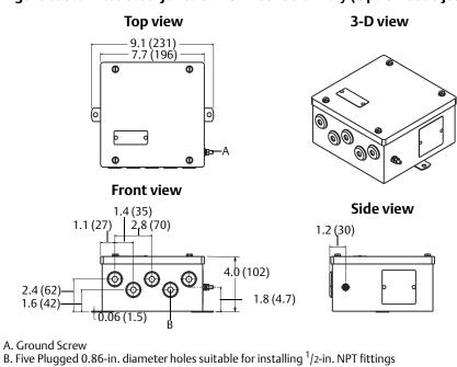
Figure 6. Stainless Steel Junction Box–Conduit Entry (Option Code JS3)
