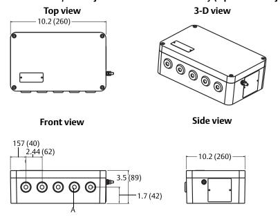
A. Five Plugged 0.86-in. diameter holes suitable for installing  $^1\!/\text{2-in.}$  NPT fittings
