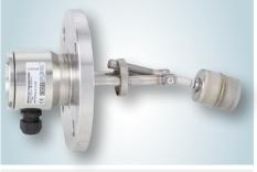
Process connection: Flange: DIN, ANSI, EN 0 ... 232 bar Pressure: -196 ... +350 °C Temperature: Density:  $\geq 600 \text{ kg/m}^3$ Material: Stainless steel, titanium Data sheet: LM 30.02
