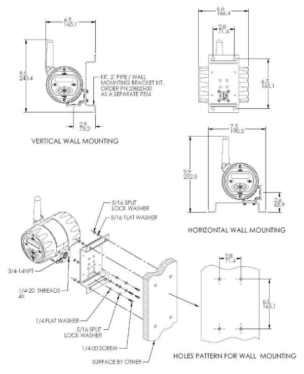
Wall Mounting Installation for 6081. Use Pipe/Wall Mounting Bracket Kit, PN 23820-00 Note: PN 23820-00 mounting bracket kit includes mounting hardware for pipe mounting only. Wall mounting hardware to be provided by customer. Only use suitable fasteners and hardware to securely fasten the bracket and transmitter to the wall surface.
