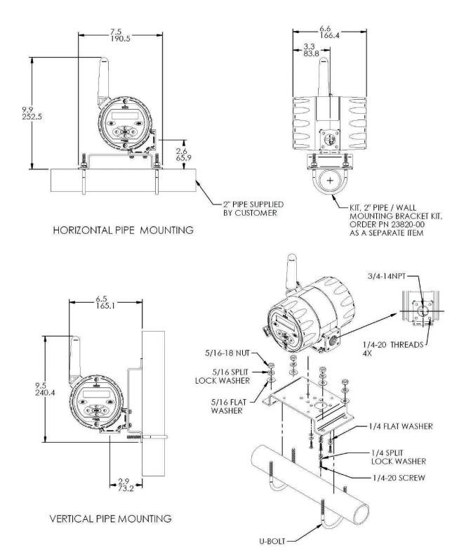
Pipe Mounting Installation for 6081. Use Pipe/Wall Mounting Bracket Kit, PN 23820-00
