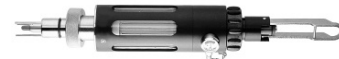
Step 1: Pressurized Mounting Assembly shown without cable protection cap. Notice the lever is in pressurized position.
