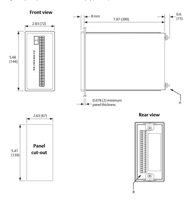
A. Panel retaining clamps (two positions)
