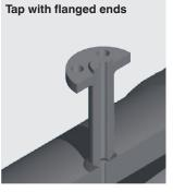
Annular chamber tap, from pipes
