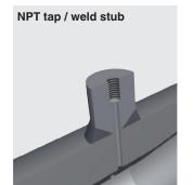
Annular chamber tap, welded ring
